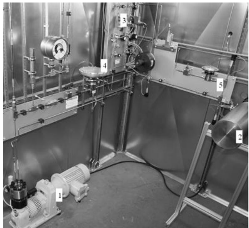
Figure 3. Some components of the hydrogen test area at the ILK Dresden: e.g. (1) – high-pressure compressor, (2) – dewar of the cryo-cooler, (3) – gas supply for hydrogen and helium, (4) and (5) – mass flow controller.
